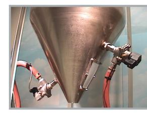
Virtually maintenance-free performance. The patented valve design utilizes only one moving part, ensuring an immediate reseal after each pulse, to prevent material feedback.
